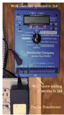
WSR Indoor Models easy and firmly mount on a stud wall and easily plug in into a wall socket. Easy connection of valve wires are shown above. WSR8 & WSR12
